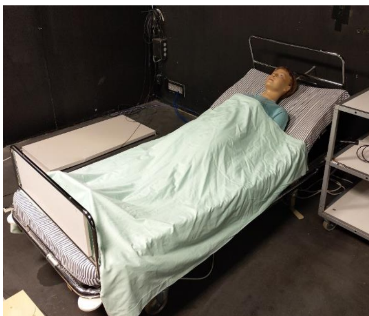
Figure 2.5. Thermal manikin lying in the bed with a duvet cover on during the thermal comfort measurements.
