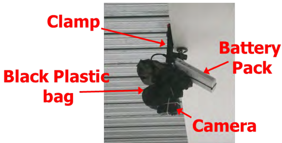
Figure 38. Example set up of a GoPro video camera.
