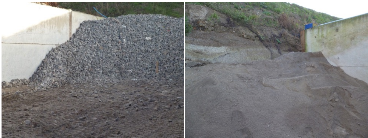
Figure 22 Once concrete has been crushed it will be sieved and sorted into different sizes and qualities
