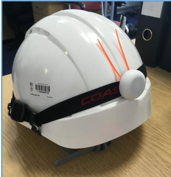
Figure 3 A UVB sensor attached to the rear of a hard hat
