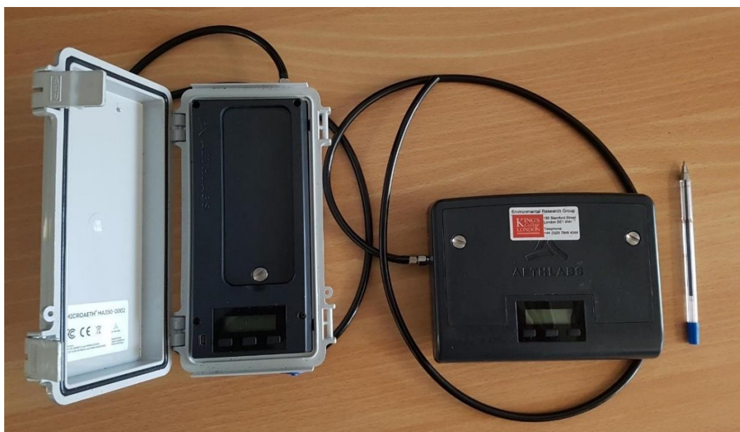
Figure 1: Picture of a microAeth 350 (left) and microAeth 300 (right)- 25 September 2019.
