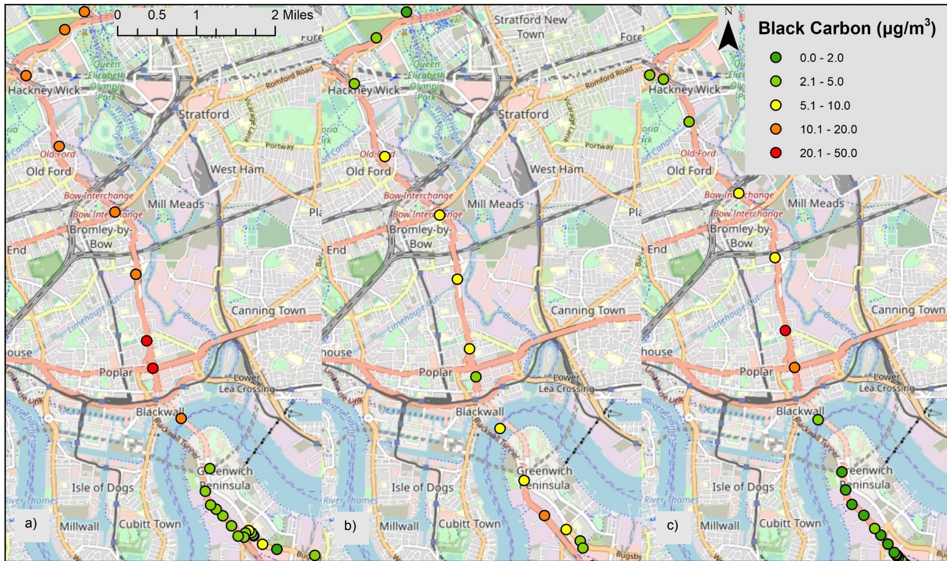
Figure 7: High BC exposure events travelling through the Blackwall Tunnel by a heavy freight driver (DEM013). a) South to north at 08:00 on 14 February 2018; b) North to south at 09:00 on 14 February 2018; c) South to north at 09:00 on 15 February 2018. Each dot represents one-minute of exposure.
