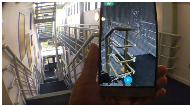
Figure 4-6 Issues in capturing scans caused by lighting and reflections
