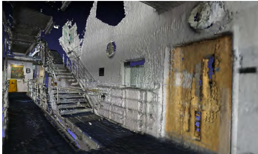
Figure 4-8 Scanning of a large area with missing mesh elements
