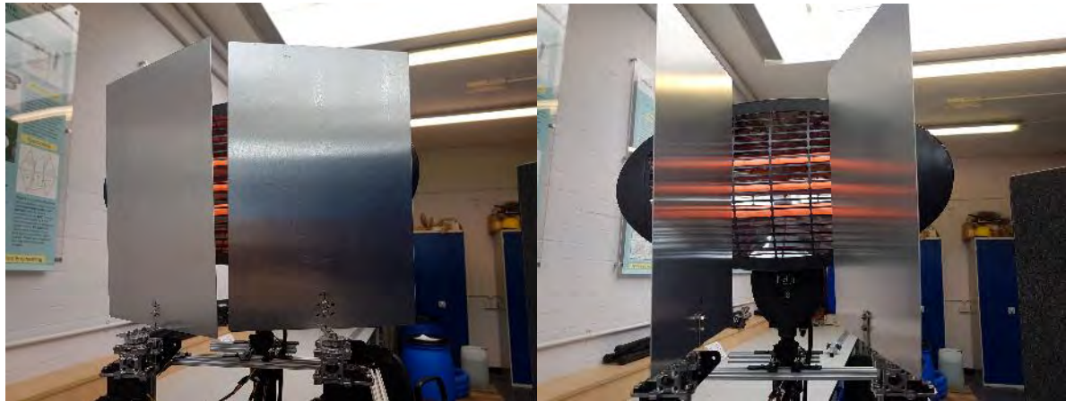
Figure 4-3 Control of heat from 2 kW infrared heater: with fins closed by default [left] and opening with Arduino control to direct heat towards user [right]
