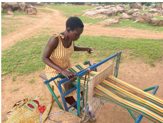
Image 4c. A weaver receives the shuttle in the left hand after sliding it through the open warp between the reed and heddle.
