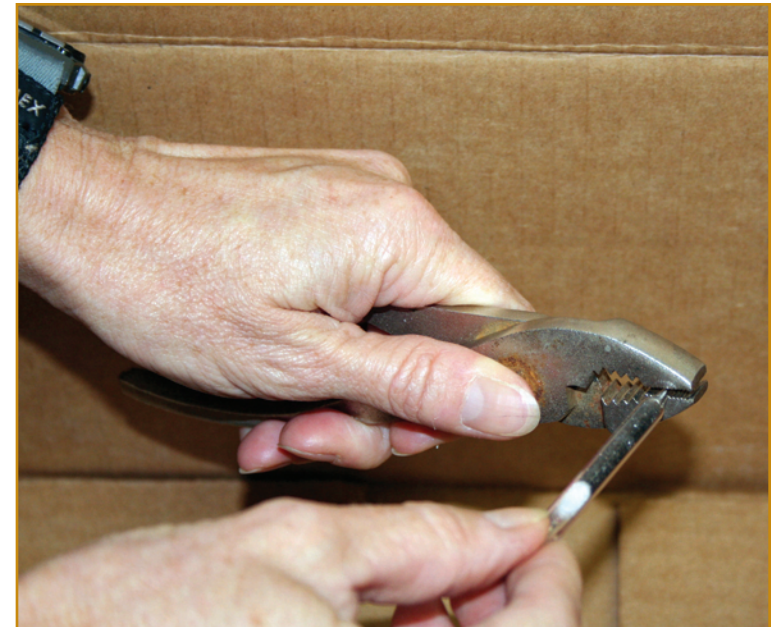
Figure 4: Just before using a tube, use a commercially available “tube breaker” (left) or pliers (right) to gently break the glass tip off each end of the tube so that air can flow through it. As a rule of thumb, break the tip at a point that will make an opening about half the diameter of the tube body. Check that both ends of the tube are open – improperly opened tubes will cause the air sampling effort to fail.
