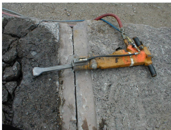
Jackhammer equipped with water spray delivery system to control dust. The water nozzle is mounted on the jackhammer frame just to the right of the chisel. Note the wet concrete on left from the water spray.
