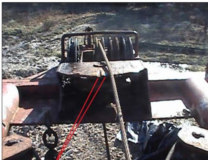
Wear marks in draw-works guard from failed line.
