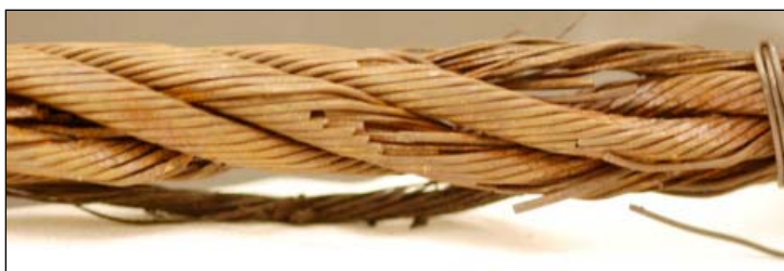
Failed 7/8" load line close-up. Note the broken wire strands.
