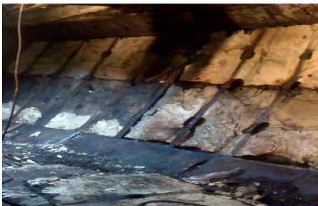
Figure 2. A shipboard confined space undergoing repair. It contains foam insulation, which can present a fire hazard.
