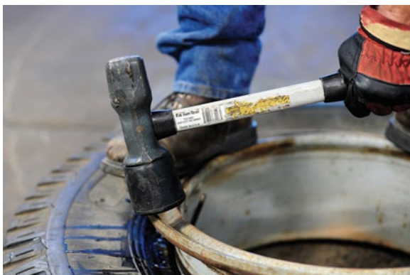
Rubber mallet setting side ring in multi-piece rim.
