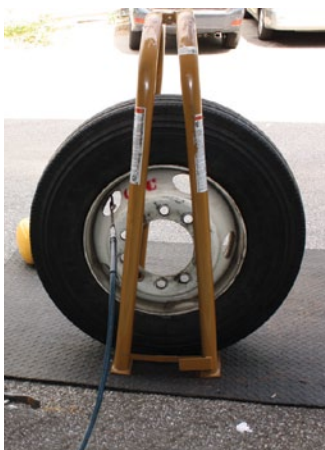
Inflating single-piece rim in restraining device.
