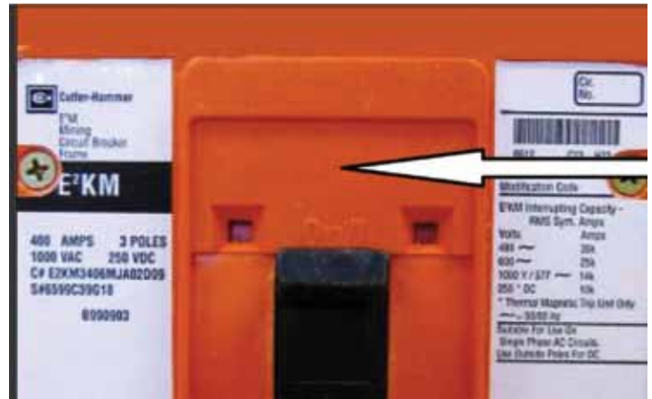
Figure 1 (Note: The arrow in Figure 1 points to an area on the frame of the suspected modified breakers that the MSHA alert notes is smooth. Originally, the E 2 K model had a grey cover and the E 2 KM model a red cover. Also, the breaker's label or frame apparently lacks the mark of a qualified Nationally Recognized Testing Laboratory (NRTL). OSHA knows of no other exterior means of identification.)
