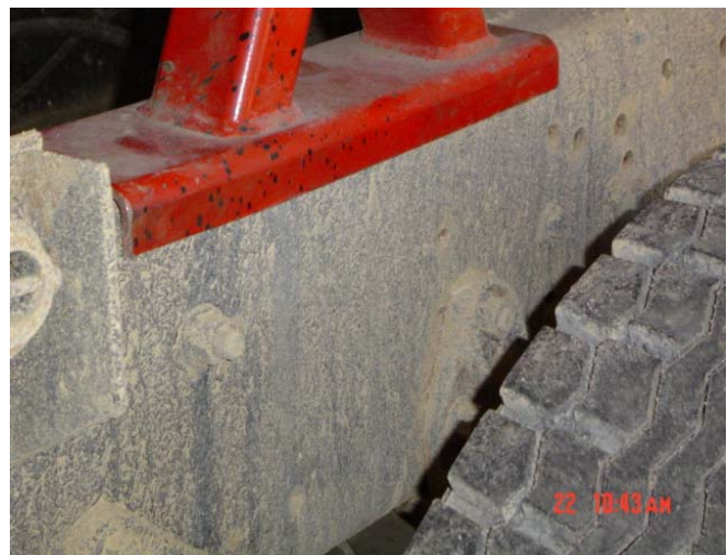
Figure 6. Truck bed brace bracket (bottom channel).
