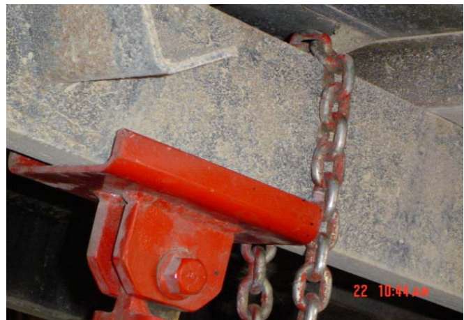
Figure 7. Truck bed brace bracket (top channel supporting dump body.)
