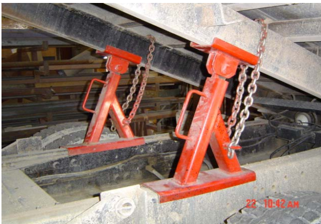
Figure 5. Engineered truck bed brace brackets.
