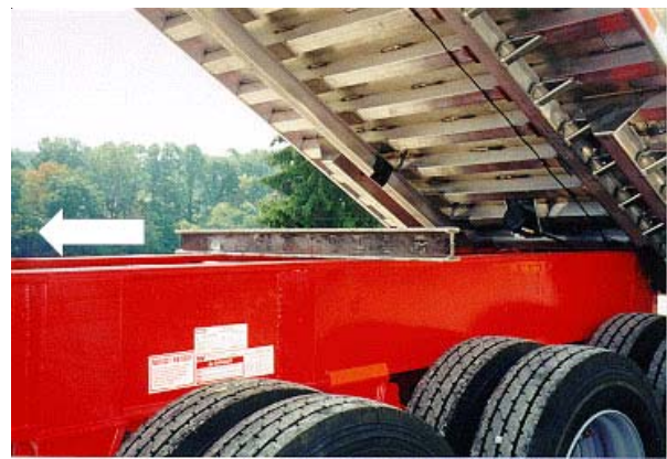
Figure 3. Shows a steel I-beam makeshift body prop: steel I-beam sits across truck frame. The I-beam is not attached to the truck frame or dump body. The I-beam could be displaced in the direction of the arrow by the inadvertent movement of the dump body or truck frame.
