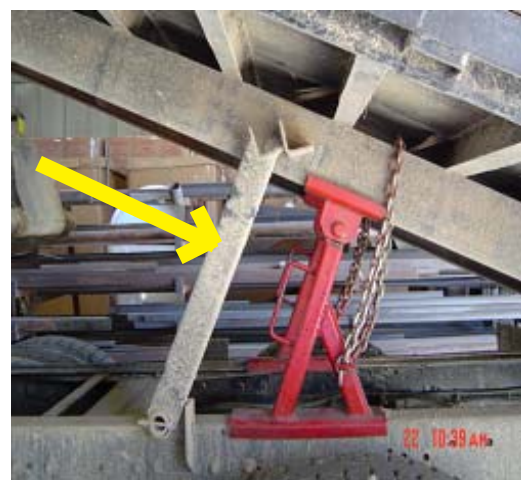
Figure 4. Positive supports are provided by dump bed manufacturers in the form of body props. Body props are non-adjustable and will support the dump body at one position only.
