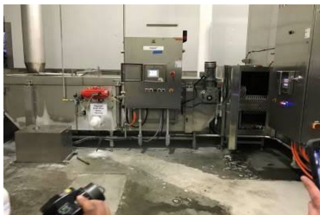
Figure 1: Six workers died from a low oxygen atmosphere when nitrogen was released from flash freezing equipment.
