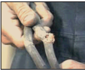
Photos showing damaged wiring that could cause an electrical fire if used.
