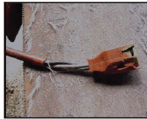
Photos showing damaged wiring that could cause an electrical fire if used.
