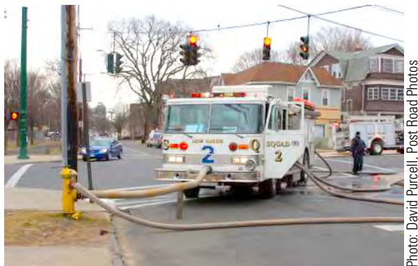
Figure 4.9. A fire hydrant located too close to an intersection can result in pumpers blocking other apparatus access.
