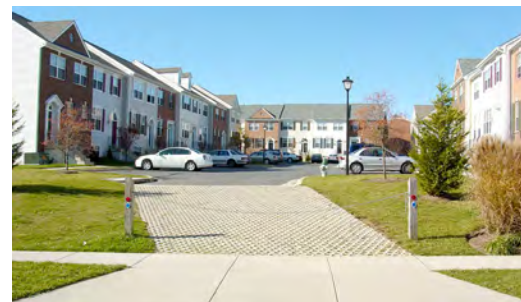
Figure 3.9. Grass paver blocks were chosen instead of paving for this fire lane. The aesthetic benefits are minimal, and the road cannot be plowed effectively.
