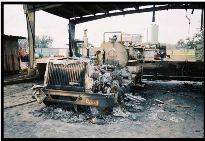
Three workers were killed and four injured in a fire resulting from a runaway diesel engine.
