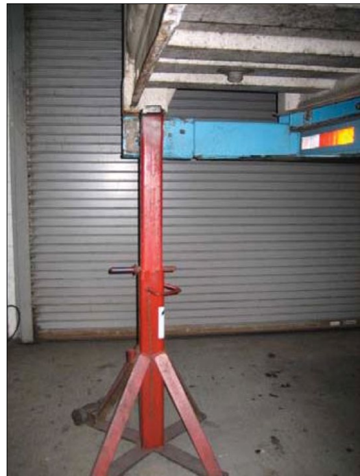
Figure 4: "Jack Stand." Note: Place the twist lock on top in the corner casting and lock in.
