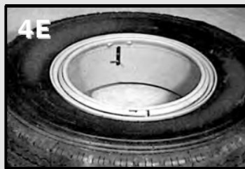
Deflating and Demounting tire from rim/wheel assembly — tube type; multi-piece
