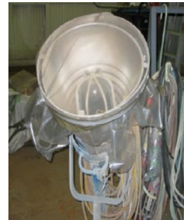
Light stand used to protect electrical cords.
