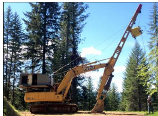
Figure 2: Excaliner with excavator pressed to the ground.
