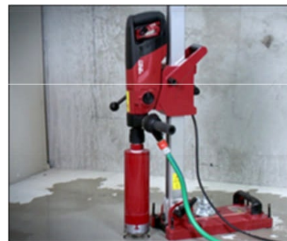
Example of a core saw with integrated water delivery system.
