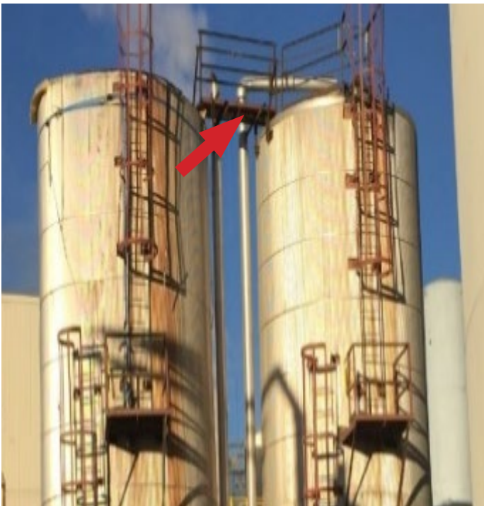
Figure 1: Soapstock tanks (red arrow shows where worker was welding when tank on left exploded).
