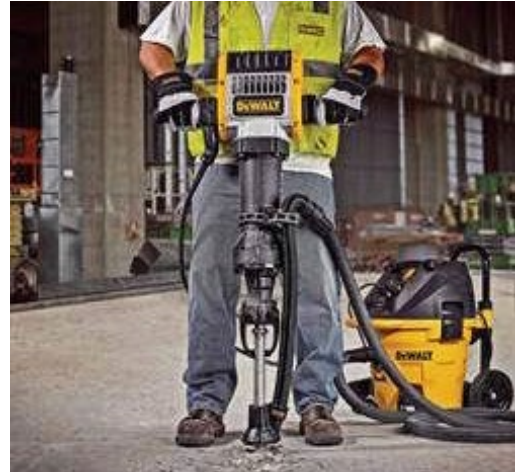
Jackhammer equipped with VDCS. Shroud around hammer connects to the vacuum on the right.
