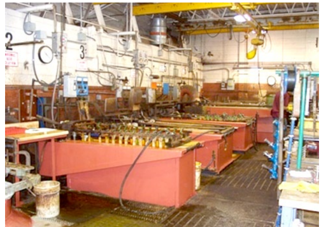
Hard chrome electroplating baths. (Photo courtesy of NIOSH).
