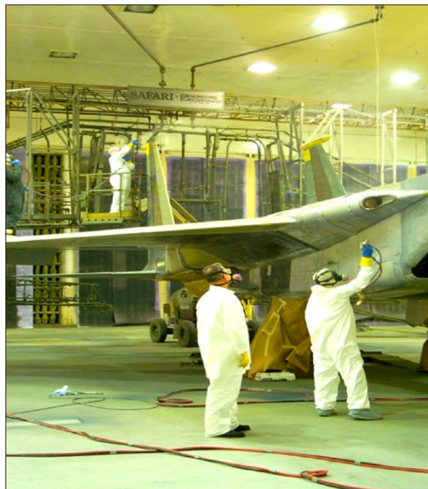
Spray painters applying a conversion coating treatment on the outside of an F15. (Photo courtesy of U. S. Air Force).
