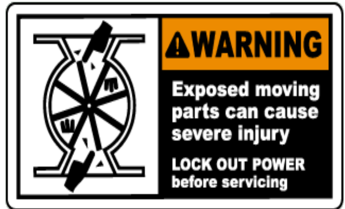
Figure 3: Hazard warning sign for rotary valve equipment. Courtesy of Conveyor Equipment Manufacturers Association
