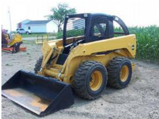
Figure 1: Typical Skid-Steer Loader
