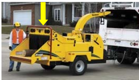
Feed control bar (in red) on top and sides with handles.
